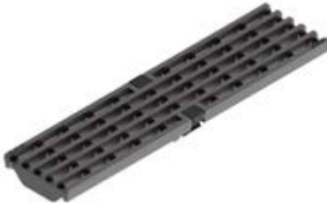
Design: Bold Bar Type: M100D Load Class: D 400 Weight: 5.7 kg Art-No.: 132088
