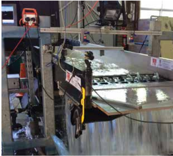
Grate intake testing based on experimental results and software developed by the UNSW Water Research Laboratory
